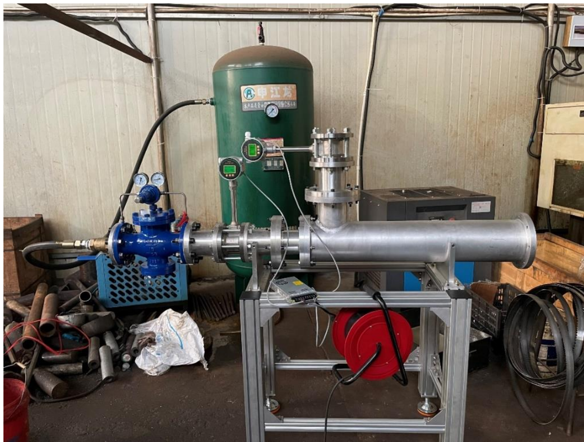
引射器测试试验台 The testbed of ejector
