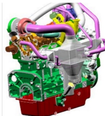
13.5L发动机有机朗肯循环系统三维图 3D view of the organic Rankine cycle for the 13.5L engine
