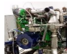
烟气管路 Flue gas piping
