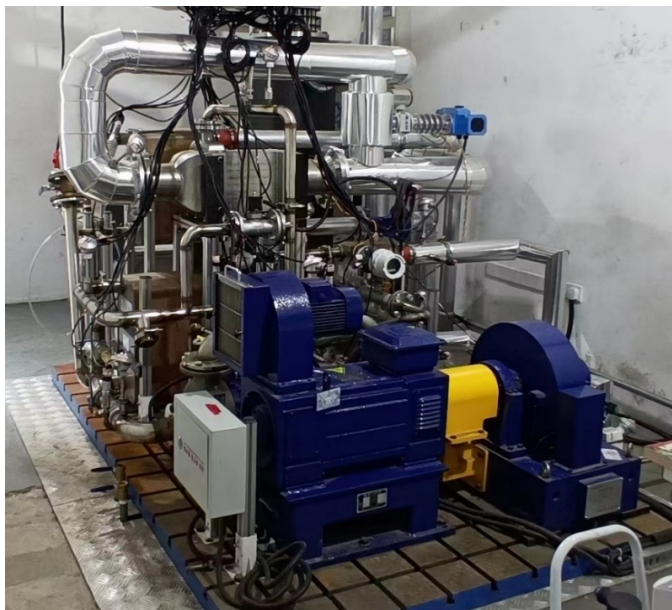
低压蒸发单级有机朗肯循环样机测试平台 Low pressure evaporation single stage ORC system bench
