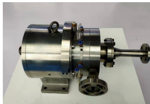
5kW级sCO 2 轴流透平(半封闭) 5kW sCO 2 axial flow turbine (semi-enclosed)
