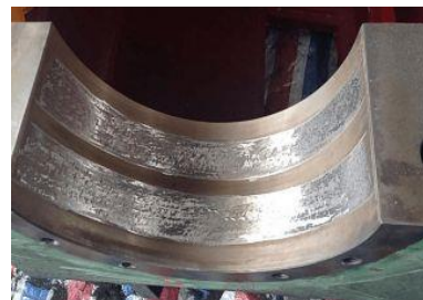
轴承磨损 (Wear of bearing)
