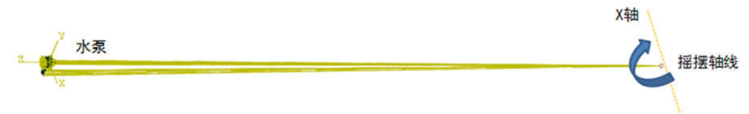
船舶纵摇状态下水泵应力计算模型 Calculation model of pump stress in ship pitching
