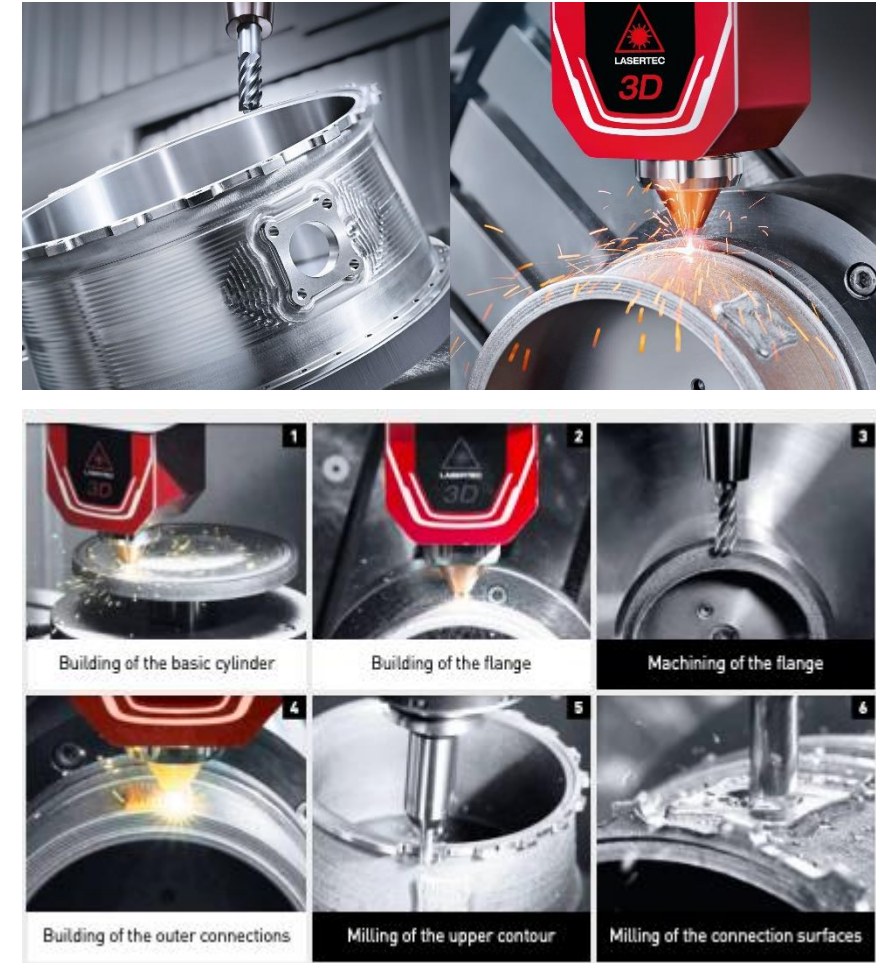
Fig. 35 A turbine case manufactured through LASERTECH 65 3D hybrid [26]
