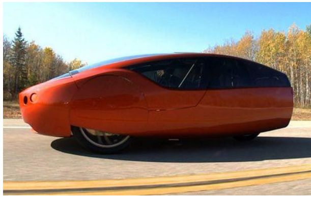
Fig. 22 Urbee Hybrid: the world's first 3D printed car [18]
