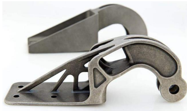
Fig. 14 Topology optimization of the aero-bracket [10]
