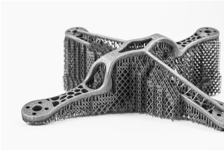
Fig. 27 Sacrificial supports in metal additive manufacturing [23,24]
