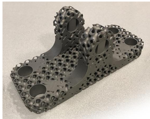
Fig. 13 Lattice topology optimization
