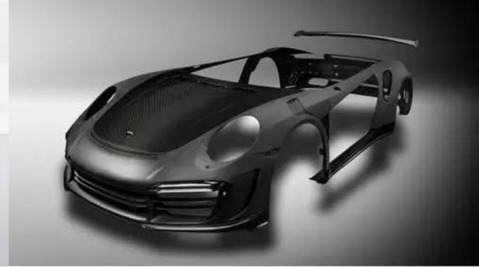
Fig. 6 Lightweight material for the car body [5]
