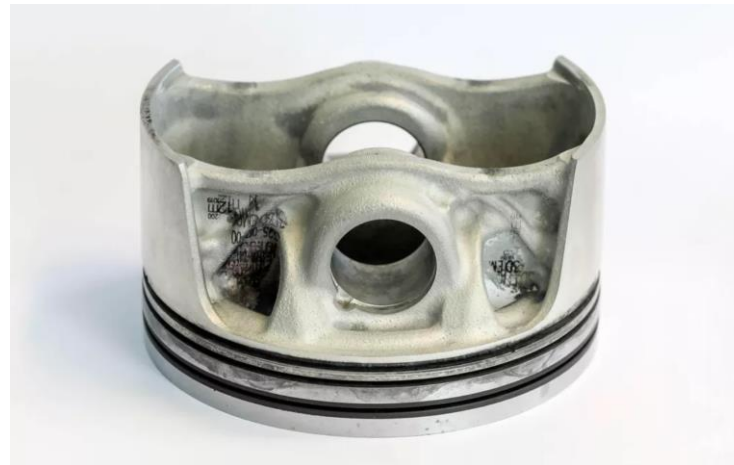
Fig. 20 Additive manufactured pistons run in Porsche GT2 RS (20% weight reduction) [16]
