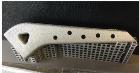
Fig. 30 Residual stress-constrained TopOpt [25]
