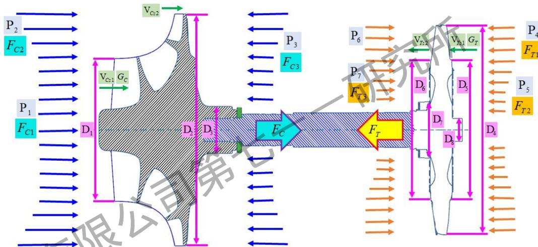
$$F_{C1} = \frac{\pi D_1^2}{4} P_1 + G_C (V_{C1} - V_{C2}) \quad (1)$$
