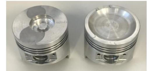
燃烧室形状对比图 Comparisons of stock and modified pistons
